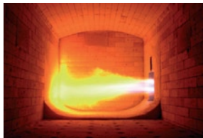
EBF – Injection burner with stoker auger
