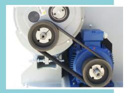
The wood-shredder works silent and poor in dust emittion. The vibrations are reduced as much as possible by the use of a V-belt and the storage on special oscillating rubber elements. Electric motors of 18.5 up to 55 kW can be choosen as required and depending on the settings of tasks. The high performance helical gear unit works with high efficiency and we ensure 2000 working hours of warranty.
