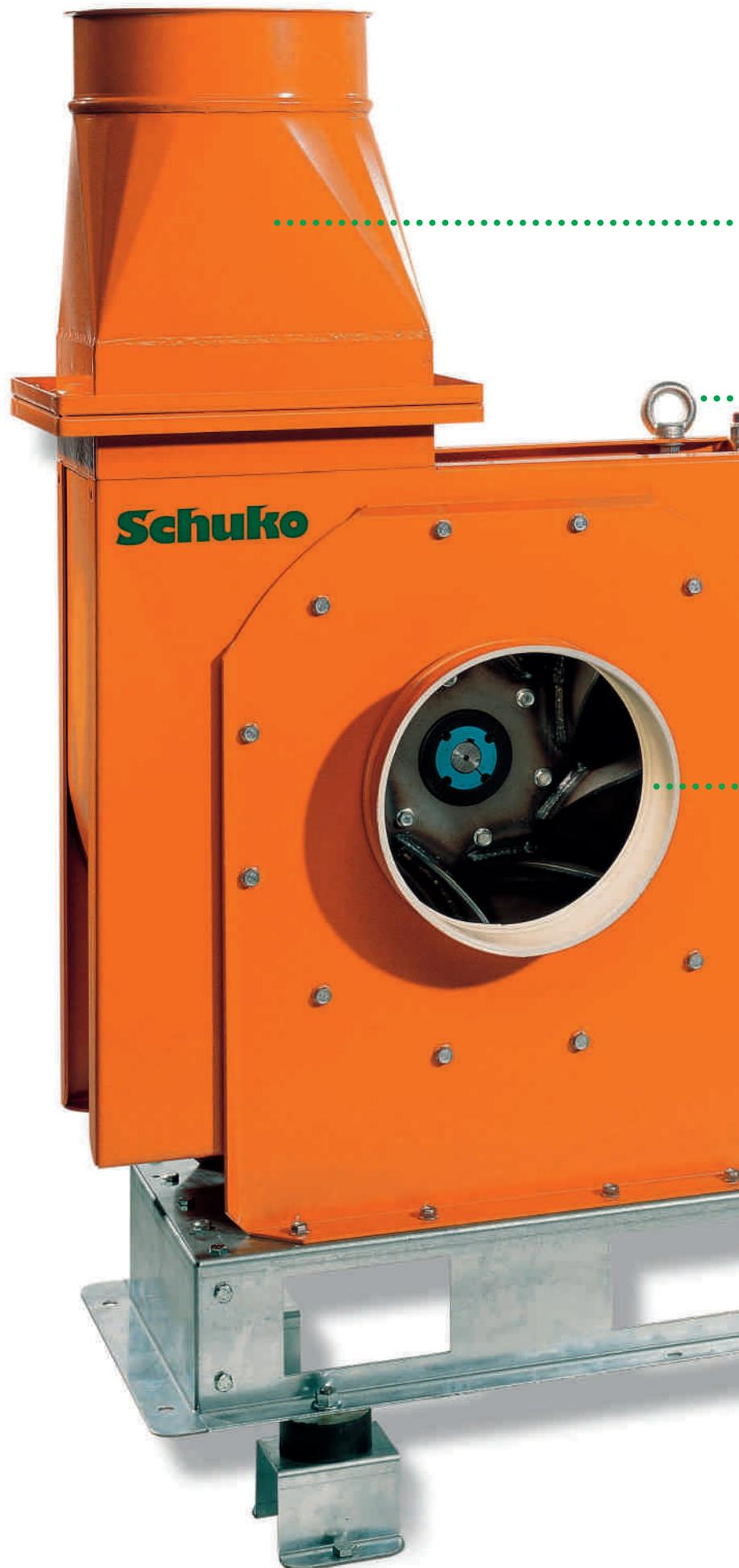
*Schuko fans are designed for single-, two- or multi-stage (infinitely variable) speed ranges. The fan housing is made of steel and welded up to form a pressure-tight structure. Suction and pressure ports belong to the scope of supply. Thus, round pipelines can be directly connected with the aid of clamps or flanges.*
